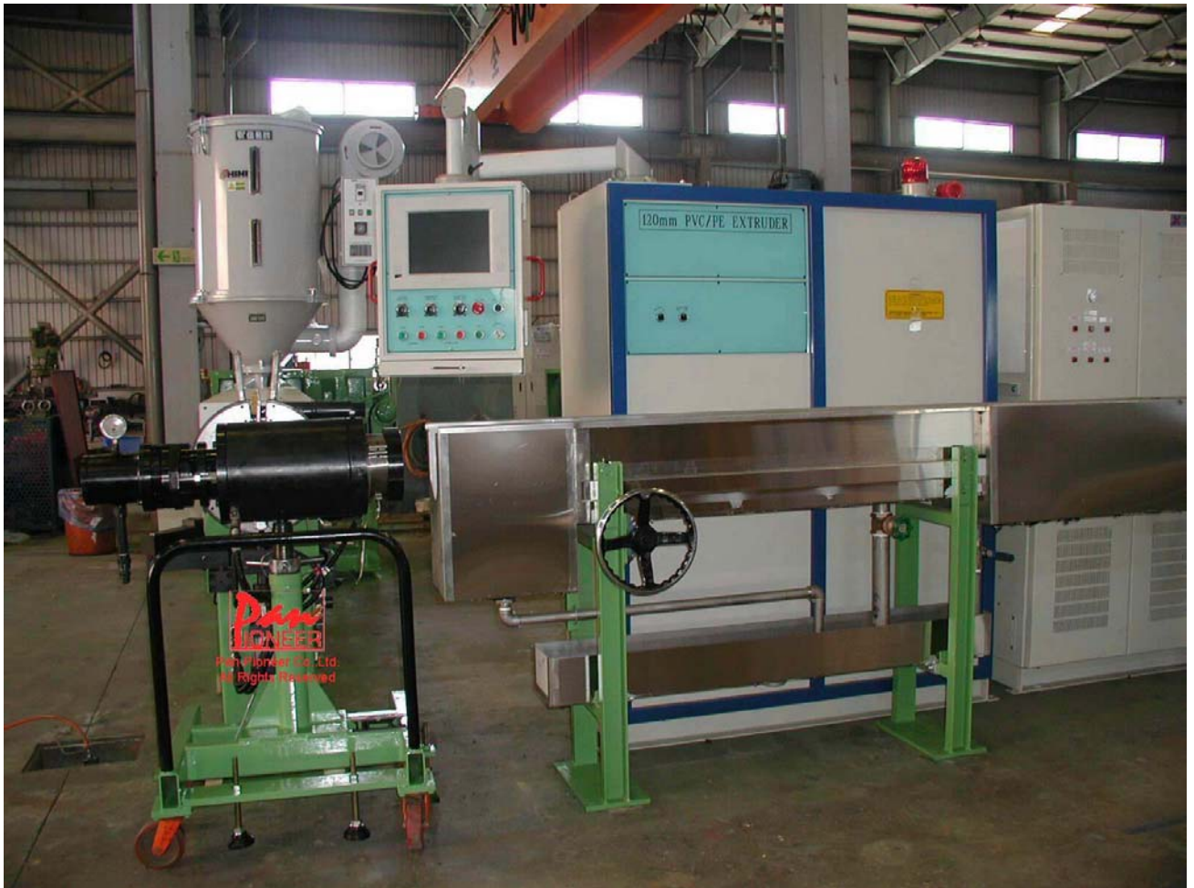
120mm Main Extruder with TFT color computer control system
