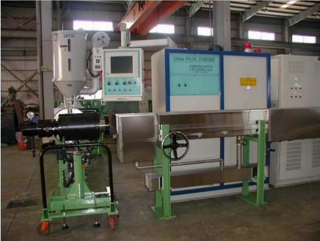
70/90/100mm Extrusion Line with Computer Control
